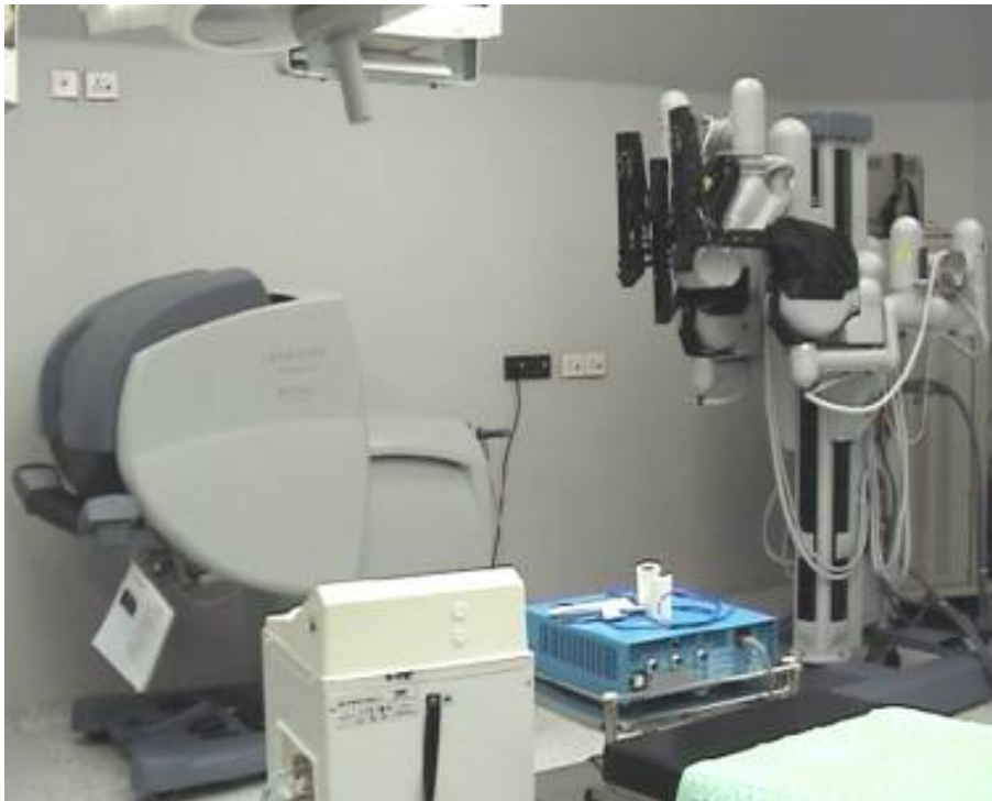
Figure 1. DaVinci Tele manipulation system- Master console and Surgical Cart
